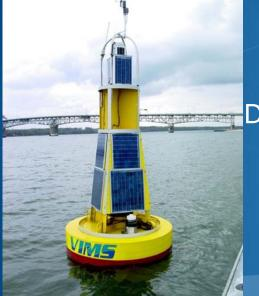
Development of Buoys and Biosensors for Remote Sampling for TMDLs
