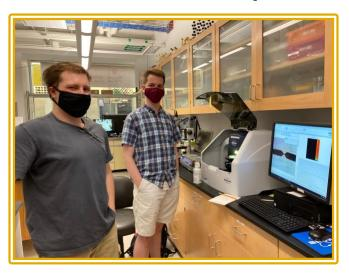
Andrew Beling (right) is working with Brennen Brown (left) on the DektakXT to analyze the flatness of copper samples and determine the need for further polishing of the samples. The samples will serve as the substrate for future atom chips in W&M's Ultra-cold AMO laboratory.
