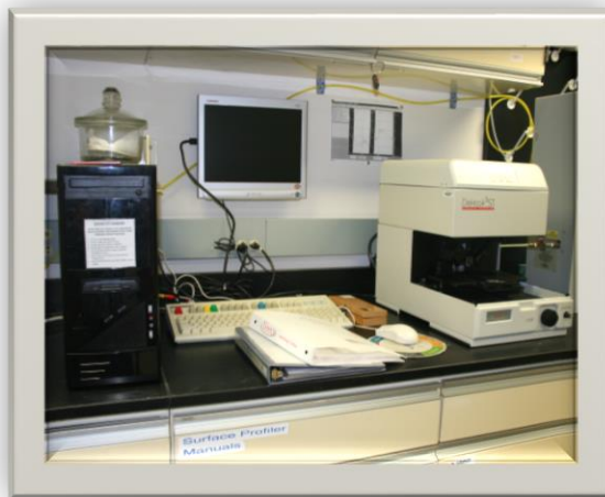
The Dektak 3 ST Surface Profiler in Lab 121 is up and running again with a new computer tower and software.
