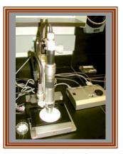
The Hirox KH-3000 is an optical microscope with digital video and imaging, which allows us to zoom and take measurements in real time. The microscope can zoom in to a maximum magnification of 7000x, in video or still images, and supplements this with a number of options for enhancing the image quality. The KH-3000 also has a
