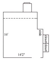
Dotted line indicates sloped ceiling. Room occupancy 2 Ceiling height 9'5" # of outlets 6 Sink yes Bathroom Facilities hall Built-in furniture no Medicine Cabinet yes Closet size 2'11"(d) x 2'5"(w) Window size 4'6" (h) x 2'3"(w) Air-conditioned yes
