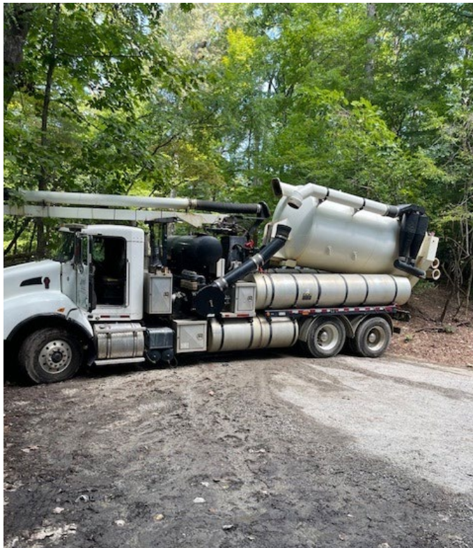
Vacuum truck in position to perform pumping operations at the BMP. Photo taken on 8/26/24.
