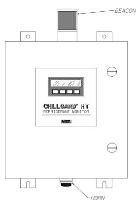
Figure 1-5. Chillgard RT Monitor with Optional Beacon
