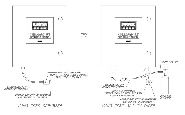
Figure 4-3. ZERO Calibration
