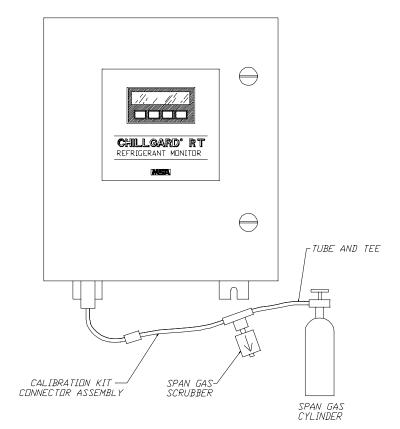
Figure 4-4. SPAN Calibration
