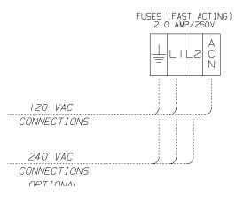
Figure B-4. Chillgard RT Relay Module Power Wiring Diagrams for 120 Volts and 240 Volts AC
