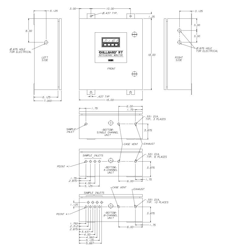
Figure 2-3. Mounting Dimensions
