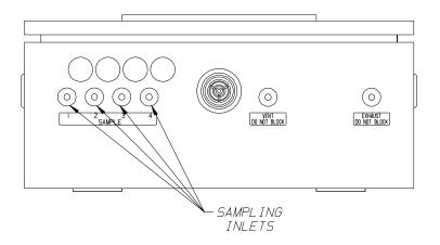
Figure 1-3. Four Point Sequencer Unit
