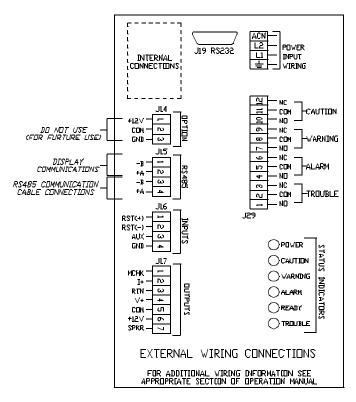
Figure 2-5. Wiring Connections
