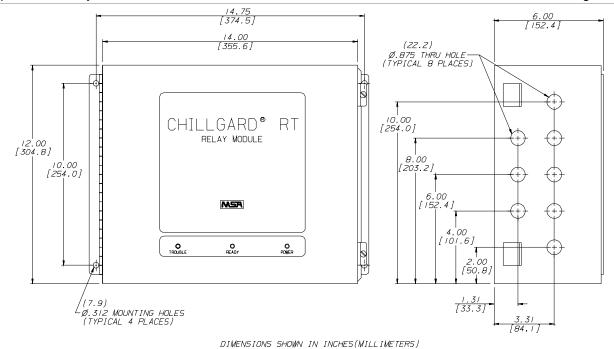
Figure B-2. Mounting the Relay Module
