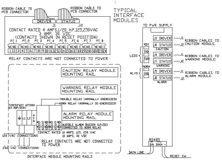
Figure B-6. Typical Interface Modules
