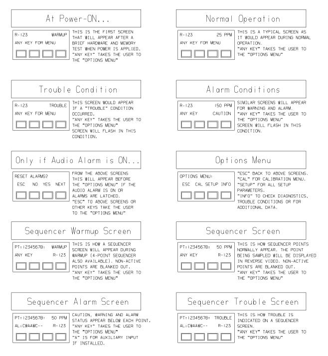
Figure 3-2. Start-up and Normal Operation Screens
