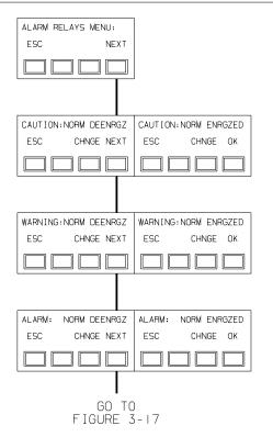
Figure 3-14 Alarm Latching Screen *Figure 3-15* Alarm Latching Screen
