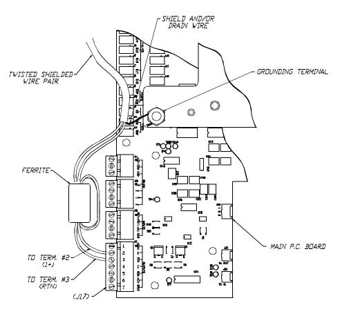
*Figure 2-6.* Ferrite Bead Installation
