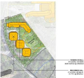
Figure 50: Conceptual Site Plan for New West 2 Housing (VMDO)
