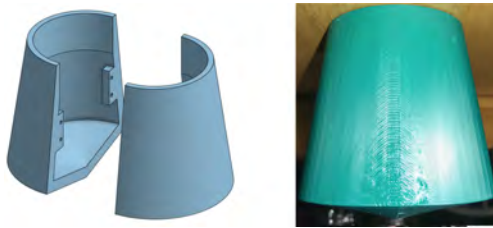
Figure 3.4: CAD design and 3-D print of the Dreidel shell shape.
