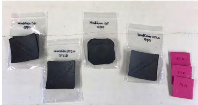
Figure 3.10: Samples of PLA and each variant of Windform to be put through ocean environmental stress tests at VIMS. Samples of ABS, not shown, were taken from fragmented prints of past shell designs.
