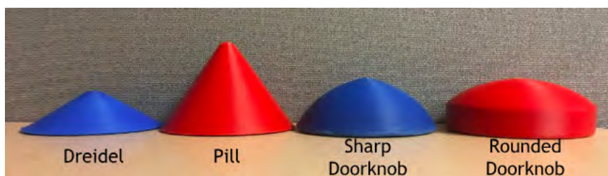
Figure 4.1: The bottom halves of the four shells under consideration at the time of the Sandbox Drop Test. Each printed at 4 in in the greatest diameter.
