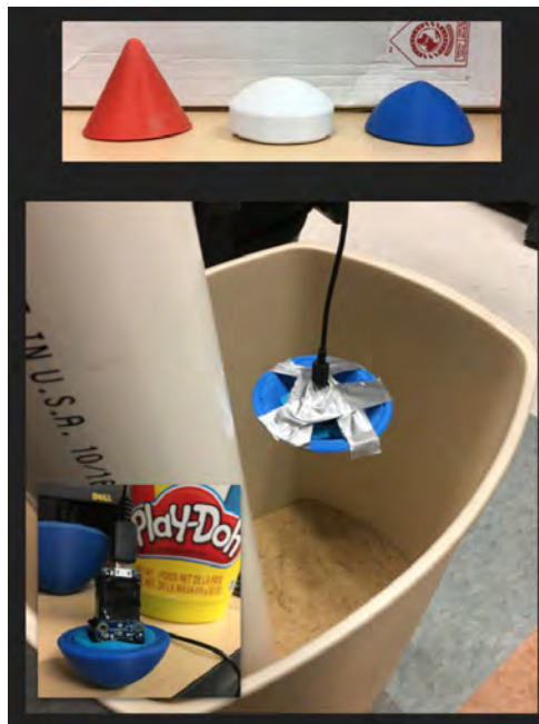
Figure 5.4: The experimental setup of the first round of the sandbox test showing the 3 shell shapes we used, and the bin containing the sand with an example of the shell shape and electronics combined together for one instance of the test.
