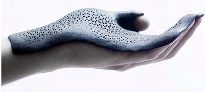
Figure 5.3: Windform GT, the material chosen to construct the outer shell of the final EDR product. It is waterproof, non-conductive, outgassing tested by NASA, and suited for cases of high impact. Image adapted from CRP Technologies [6].
