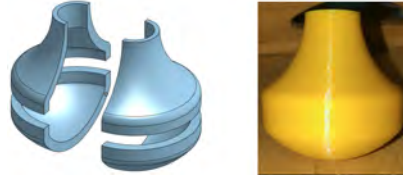
Figure 3.2: CAD design and 3-D print of the Doorknob shell shape.
