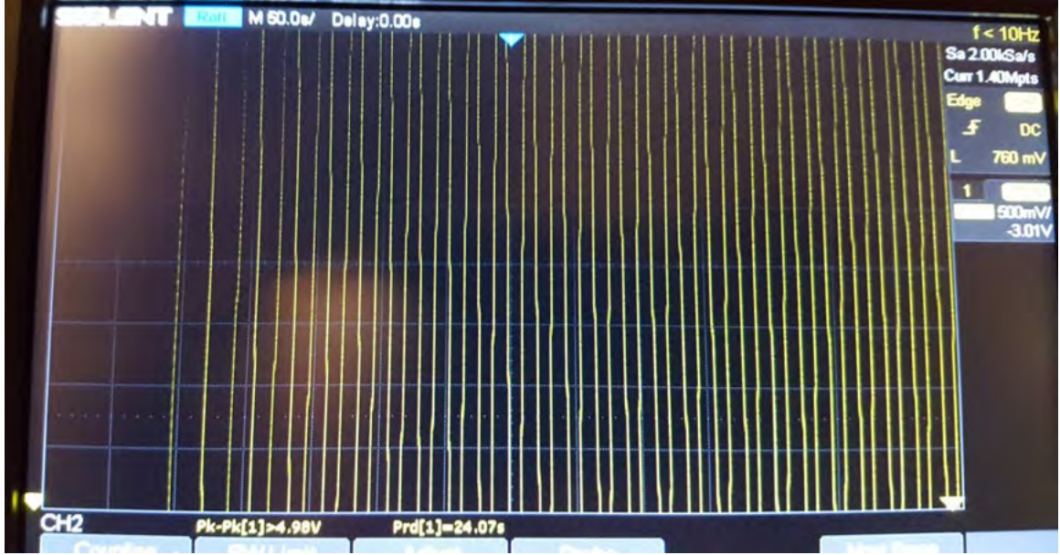
Figure 3.4: Poor PID Feedback Convergence: This is an example of a poorly tuned PID loop. Temperature is on the left axis, time is across the bottom. Over time, the system is not stabilizing, so operating the laser with the intent of having minimal or no mode hops is an excersize in futility. (Temperature is on the left axis, time is across the bottom)
