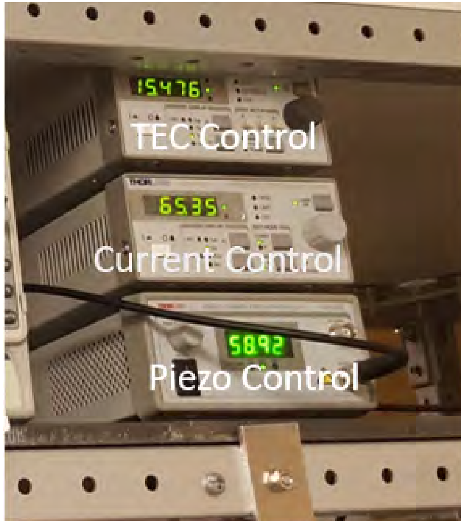
Figure 2.2: Control Boxes: The laser uses three controllers to operate, and also requires a feedforward scanbox, which was not in use at the beginning of the year. The top device is the the TEC controller, which is responsible for keeping the laser at a constant temperature. The middle device is the laser current controller, which changes the input current to the diode and can also be used to make small adjustments the output wavelength of the laser. The bottom device is the piezo voltage controller, which is used to control the input voltage to the piezo mount.
