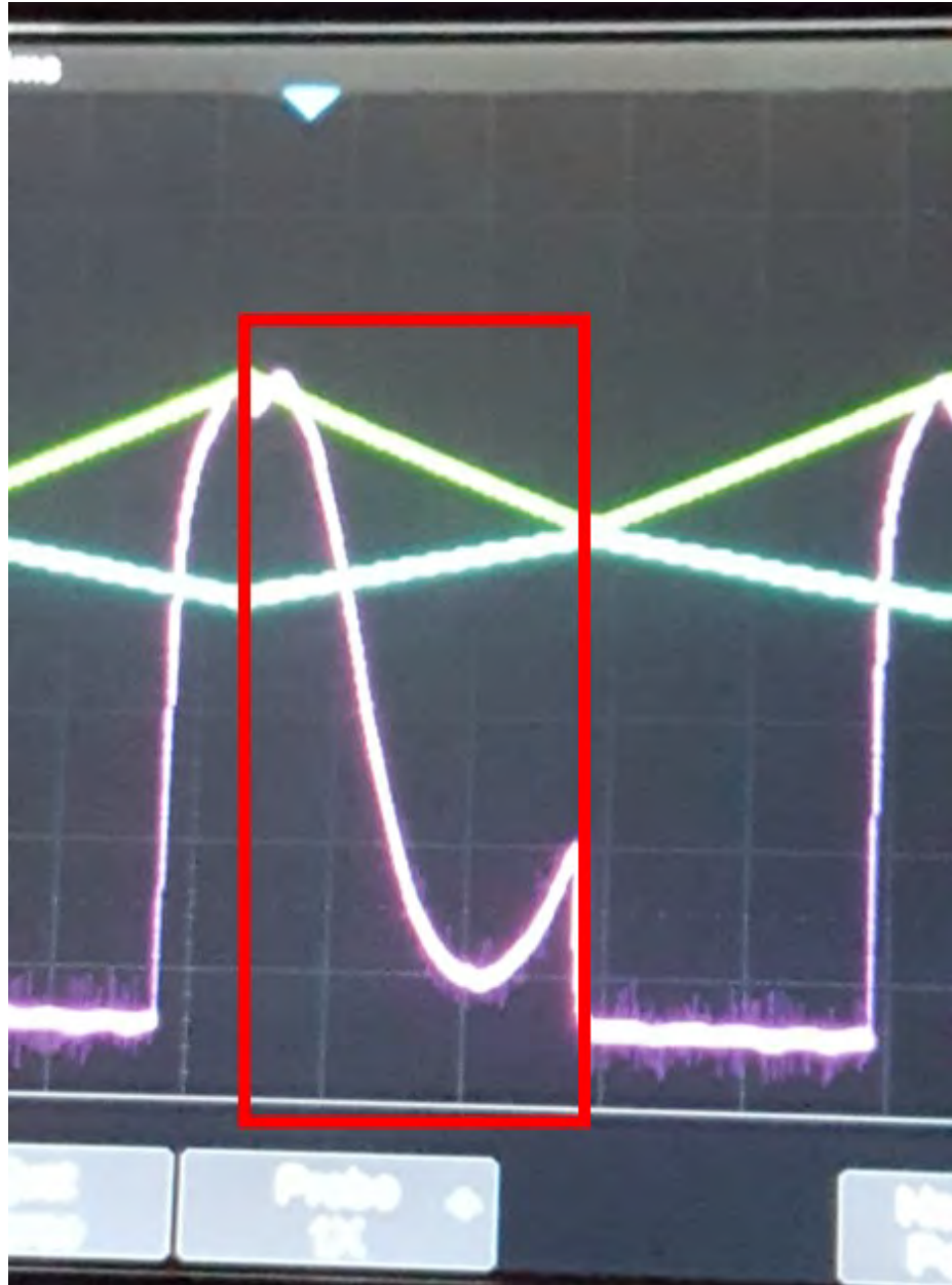
Figure 6.3: Initial Larger Scan Range: Taken on the same day as Figure 6.2. The red rectangle highlights the full scan range. Here, the range is clearly a half of one peak and the start of another, which is almost as large as the max range found in Figure 6.1. Unlike in 6.2, the scan is undergoing a one direction mode hop. There are a few variables that can cause this, and we did not take the time to isolate what the primary cause is.
