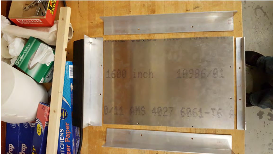
Figure 4.1: Unassembled Control Platform: These are the basic pieces of the control platform. The sides and back use the same sized L-brackets, while the front uses a smaller L-bracket to allow access to the controls on the piezo voltage controller and the laser current controller on the bottom of the stack.
