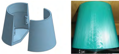
Figure 3.4: CAD design and 3-D print of the Dreidel shell shape.
