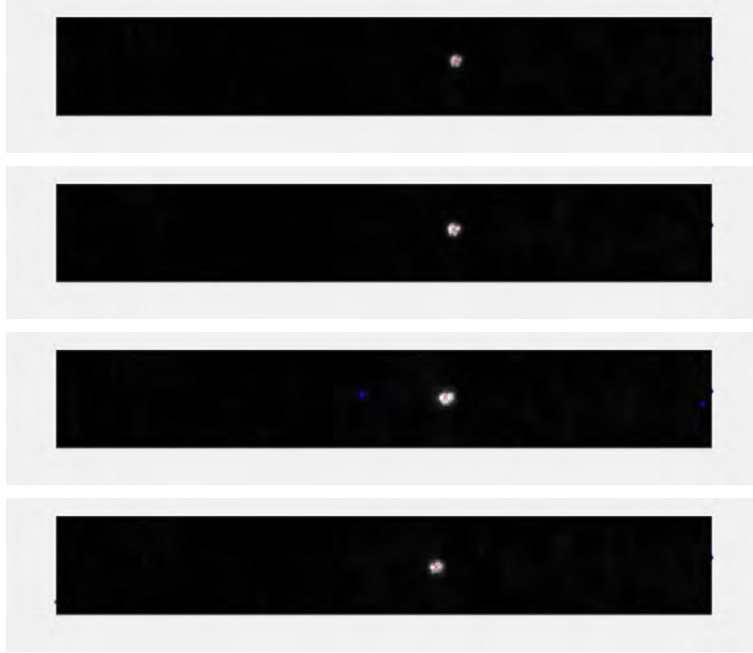
Figure 21: These frames show the centroid value for a region of a given area and how the centroid tracks over a number of frames
