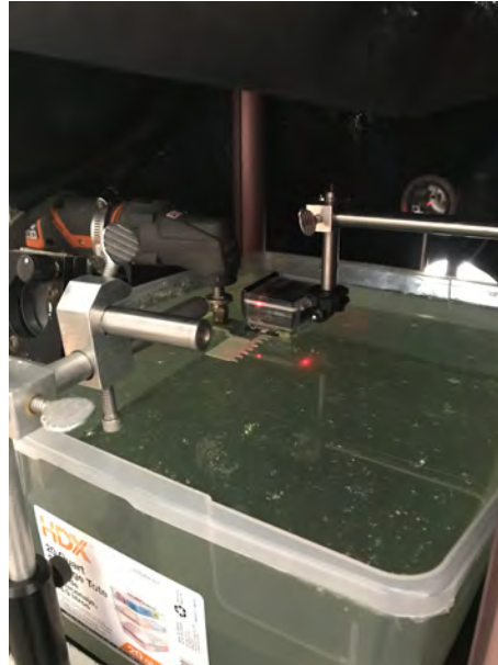
Figure 15: This image shows the yellow rosin particles that were too small to break surface tension. Those too large to be neutrally buoyant naturally sink, while the neutrally buoyant particles drift submerged at various levels in the fluid.
