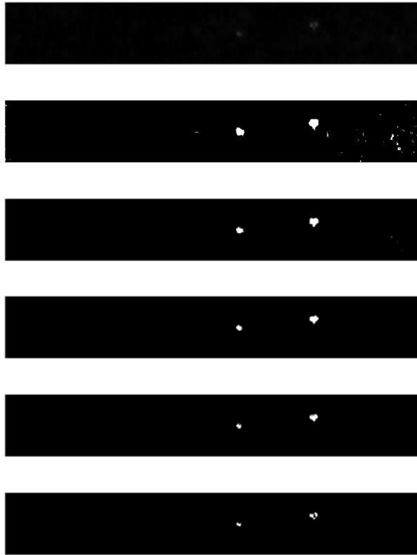
Figure 19: The top image is the gray-scaled data from our video. The subsequent pictures are threshold values in increments of 5 starting with a value of 10. While noise cancellation occurs by 20, a value closer to 25 was chosen to optimize the algorithm.
