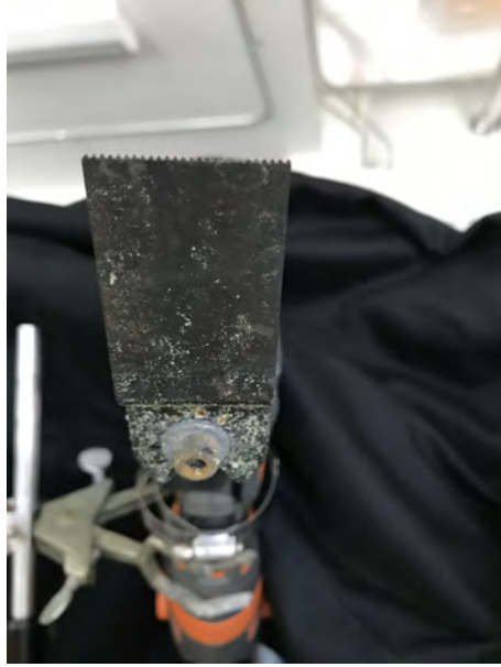
Figure 16: This image shows the wood blade we used in the experiment. Its dimensions were similar to those of the saw blade used by experimenters in the past to cut algae.
