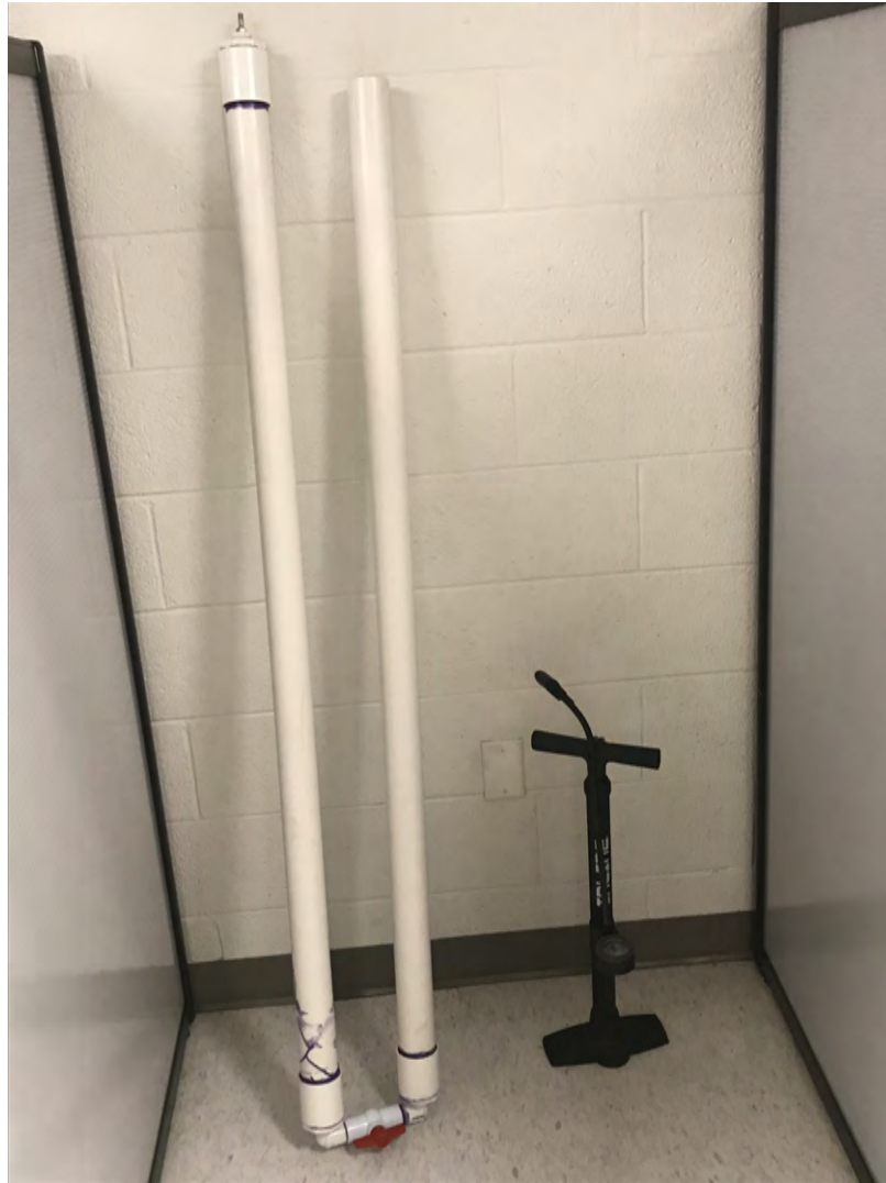
Figure 5.12: This is the air cannon used in the lateral launch tests. Next to it is the bicycle pump used to pressurize the closed chamber for each launch.
