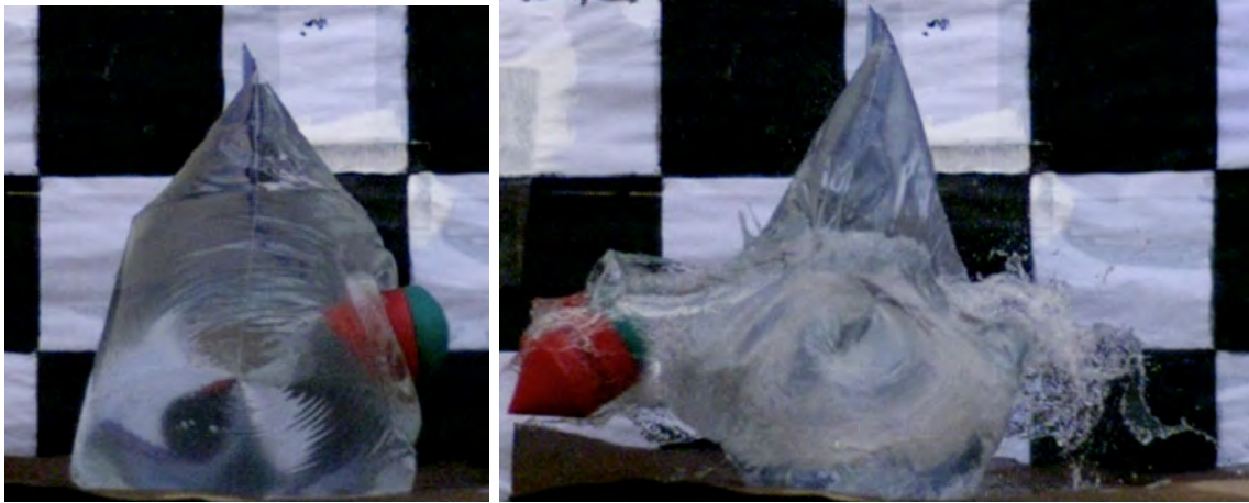
Figure 5.13: Here are still frames of the dreidel-pill miniature shell shape piercing the water bag target. Taken with the Edgertronic SC2+ slow-motion camera.
