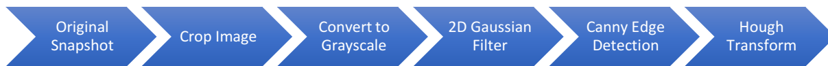
Figure 3.1: This flowchart summarizes the order of imaging methods applied to each picture.
