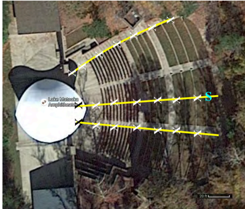
Figure 3: Speaker placement, noted by the blue "S", and audio recorder placement for the Technomad Berlin 60/40 testing. The lowest line of recorder placements were denoted "Recorder 1" in audio recordings, the middle row "Recorder 2", and the upper row "Recorder 3". Image courtesy of Google maps.
