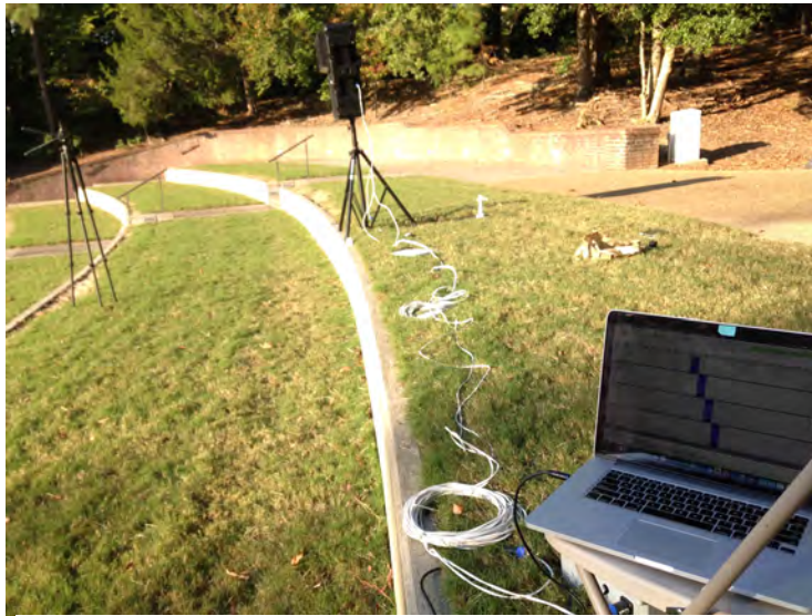
Figure 2: Experimental setup including the first speaker model, the Technomad Berlin 60/40, with Recorder 2 and the laptop from which the audio file was played.
