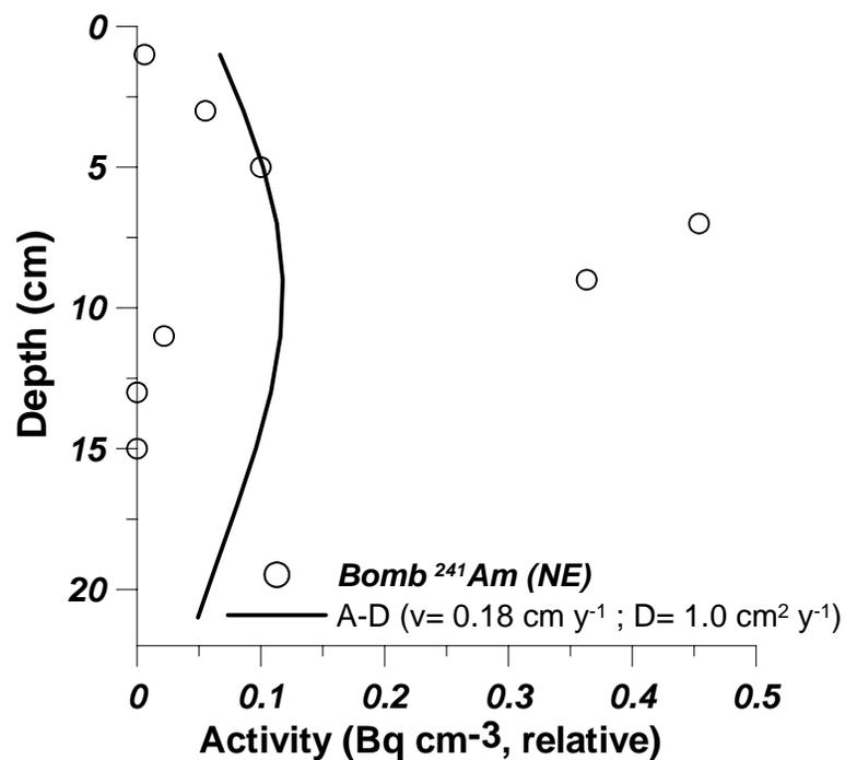
**Figure DR3.** Dynamic numerical model simulating the weapons fallout profile at a pit in NE using the best fit  $D$  derived from the steady-state  $^{210}\text{Pb}$  A-D model (Figure 2, Data Repository Figure A2). The model itself is similar to that described in Figure A3, although we use input data measured in New York from 1956-1975 (U.S. ERDA, 1977). This simulation shows how poorly the traditional A-D model describes our data in surface soils in NE.
