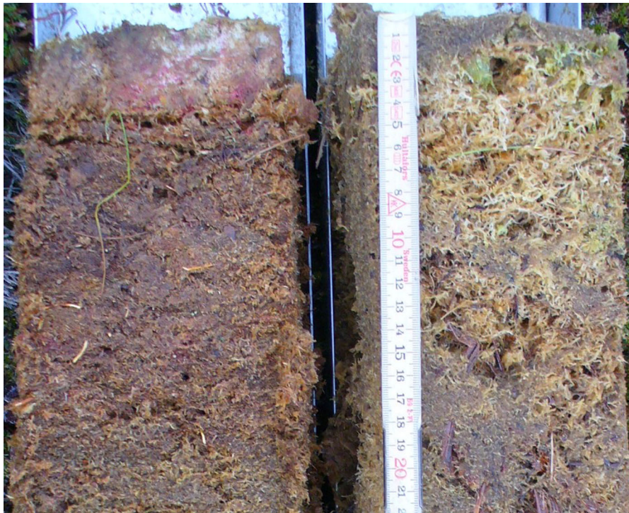
Fig. 3 Core F1c and S1c from Rödmosamyran representing fen peat ( left ) and sphagnum lawn ( right ). Note the visible difference in the fragmentation and degree of decomposition between the two cores
