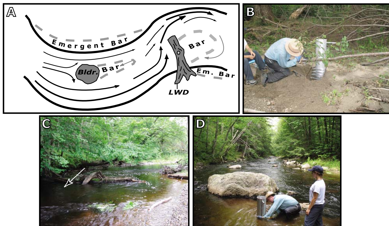
Figure 2. (a) Conceptual model of sediment bar location and formation with respect to in-channel and emergent channel features (LWD, boulders, sinuosity, etc.) along with generalized flow vectors. Photographs of (b) the coring device and metal slots used to partition 5 cm depth samples, (c) perpendicular woody debris (LWD-10.7) and associated depositional eddy (arrow) where the core was taken (downstream flow is also in the direction of the arrow), and (d) sediment storage associated with a boulder (B-9.1) in the supply-limited reach.
