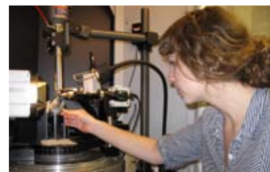
Ashley Butland '10 uses the x-ray diffractometer to look at how Hg and Zn complex with a variety of ligands.
