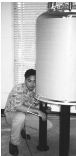
A Varian installation engineer purges the magnet dewars with nitrogen gas prior to the initial liquid nitrogen and helium fills.
