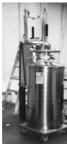
The magnet is shown here being filled with liquid nitrogen.
