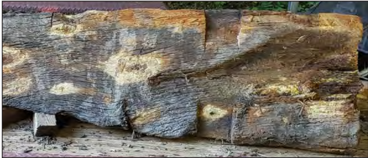
Figure 6.33. Top view of the forefoot knee showing rebates for futtocks.
