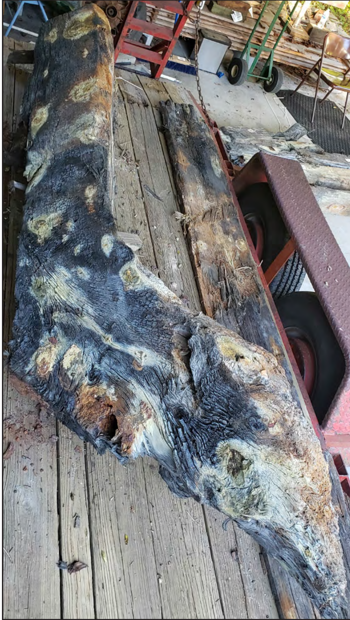
Figure 6.30. Forefoot knee starboard side looking aft.
