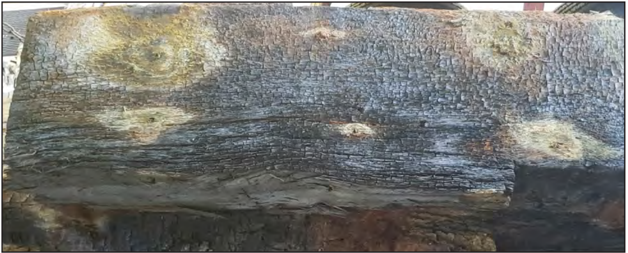
Figure 6.35. Spike pattern associated with hull plank attachment.
