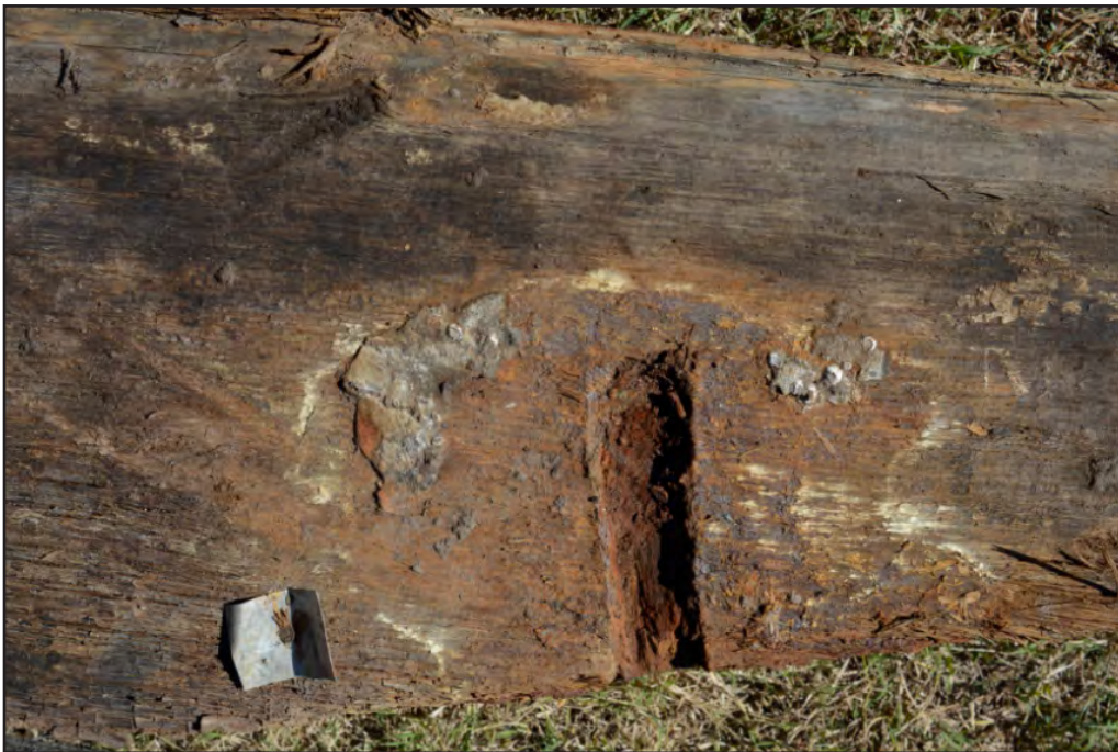
Figure 6.18. Recess for the keel scarf fishplate.
