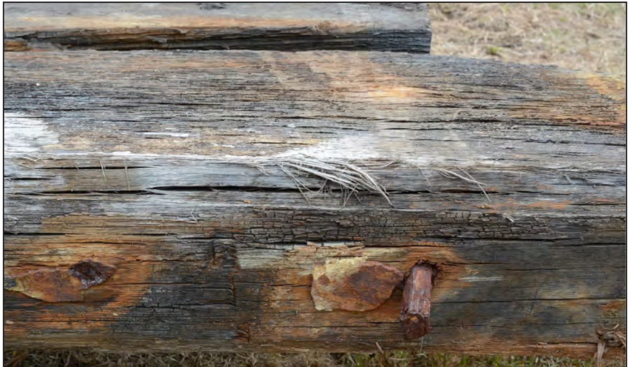
Figure 6.20. Remains of a square bolt driven through a round hole drilled into the keel.
