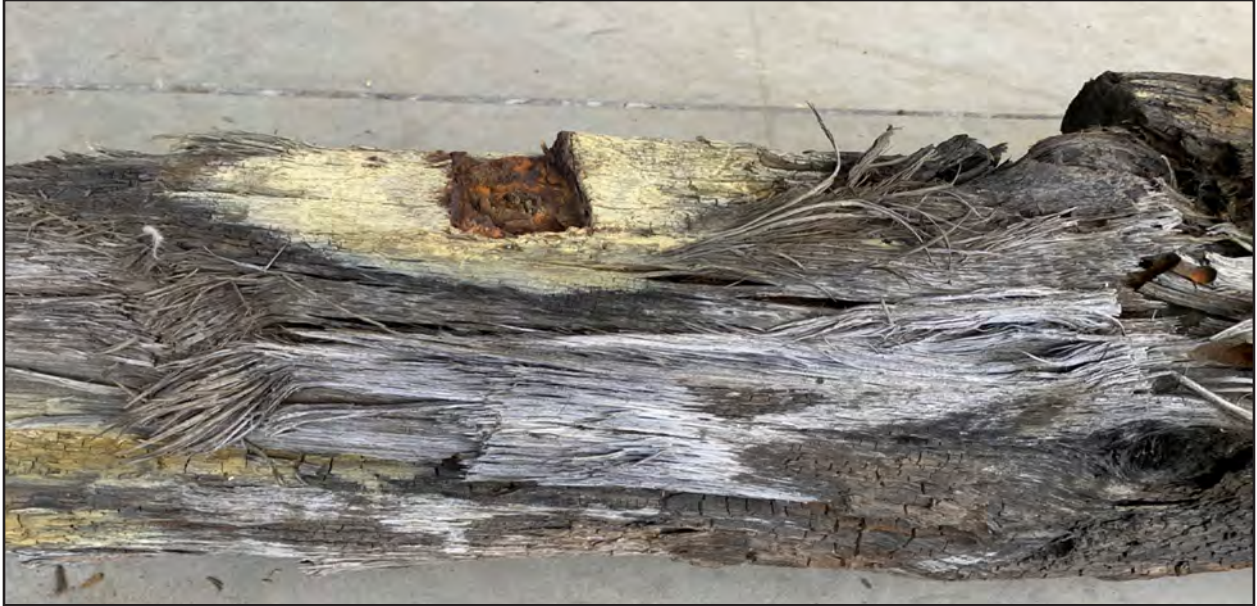
Figure 6.24. Rebate for fishplate at the scarf on KL-2.
