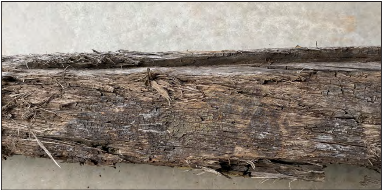
Figure 6.25. Shallow rabbet in top of KL-2 section.
