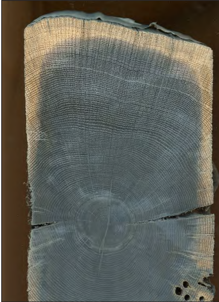
Figure 5.1. Cross-section of the keel timber 1 sample. The dimensions of the portion shown here are 26 x 18.5 cm; the whole sample is 41.5 x 18.5 cm. Note the same rings running along the upper edge, and suggestion of a slightly different ring color of the outer seven rings. The outermost incomplete ring on this sample dates to 1814, but all rings contain tyloses so at least the outer four to six rings are missing. Note the overall increase in rings widths from pith to outer rings, a normal phenomenon of closed-forest tree growth, where rings become larger as the tree is increasingly exposed to sunlight. The darker color in most of the sample is due to age and use in a vessel but may be caused partially by any substance used to waterproof the wood.
