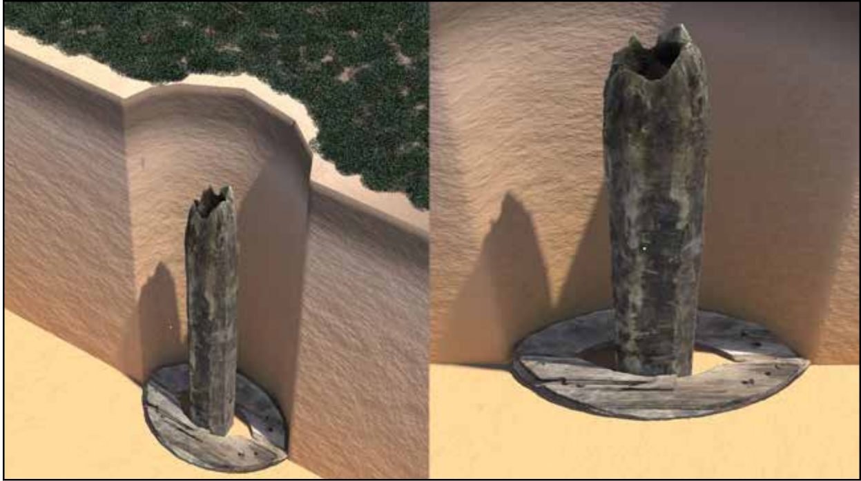
Figure 4.54. Rendering of mid-eighteenth-century lift pump stock/well at Armstrong-Rogers Site, Delaware. Note intake holes near bottom of pipe (Blondino and Gonzalez 2016).
