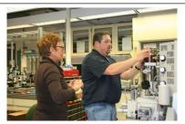
Olga was able to observe and assist Hitachi service technician Robert Harrington during the repair of the FE-SEM. Once the replacement part was ordered and installed, the FE-SEM was back in service after the vacuum was reestablished.
