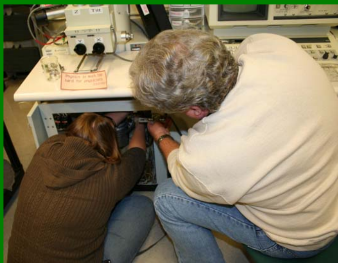
Natalie and Richard did repair work on the SEM when a vacuum hose was found to be leaking.
