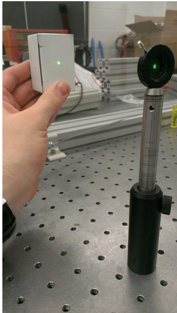
Figure 11: This shows the resulting laser beam after it has passed through two nearly closed irises.
