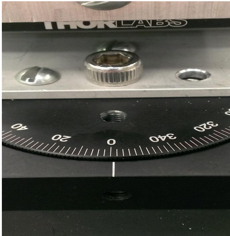
Figure 13: The alignment angle. At this angle the laser will reflect back onto itself when it reflects off of the center of the mirror.
