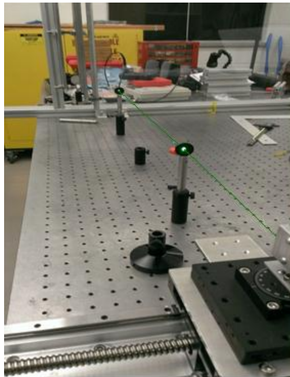
Figure 10: This figure shows the two irises used for alignment in the laser table. The path of the laser beam has been simulated.
