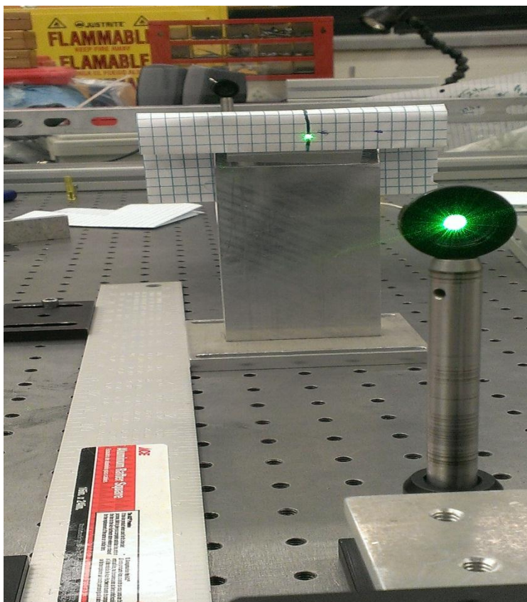
Figure 14: This shows the set up for the target. The laser is shown striking the back of the target to mark the center line. The center line was continued onto the front of the target. When the laser reflects off of the mirror, the target is moved along the y -axis until the reflected laser strikes the same point on the front of the target.
