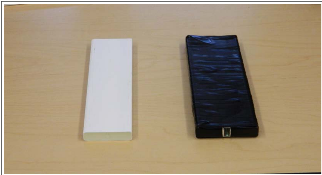
Figure 2: Left: Plastic Scintillator w/ \text{TIO}_2 . Right: Light-Tighted Scintillator w/ WLS Fiber [9]
