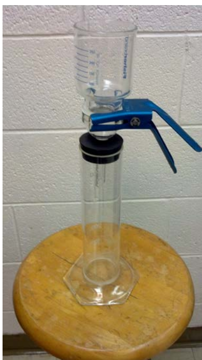
Figure 21: Apparatus used to flush diatoms with hot hydrogen peroxide.
