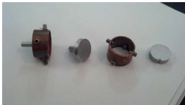
Figure 22: Modified sample tabs for imaging with both SEM and AFM. The assembled tab is on the left, and the disassembled components are on the left.
