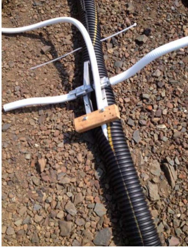
Figure 5: The “long horn” built as a tool to insert cables into the corrugated tubing.
