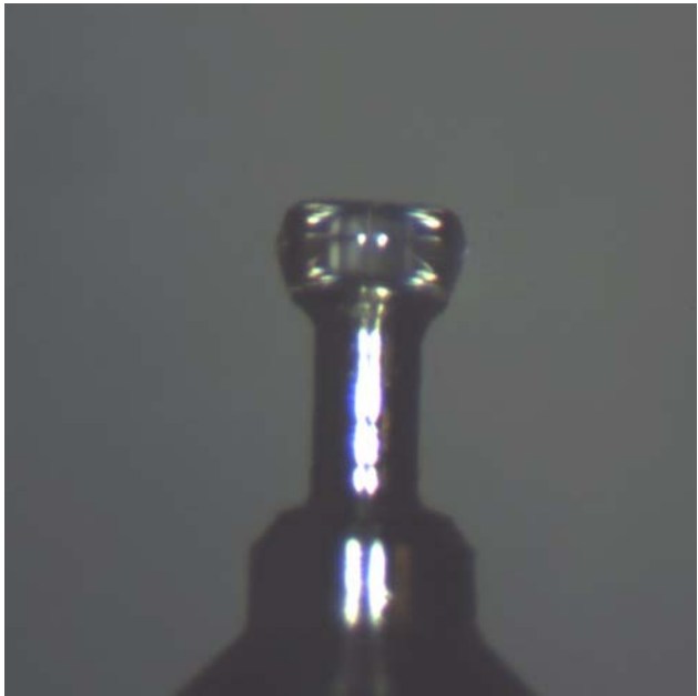
(c) A Potassium Lithium Niobate WGMR, 0.66mm in diameter (Polished by JPL, Q \sim 10^7 )
