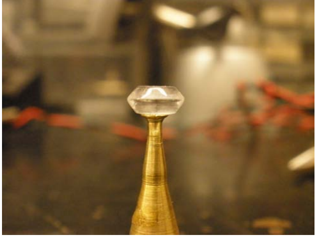
(a) A Calcium Fluoride WGMR, 7mm in diameter ( Q \simeq 1 \times 10^7 )
