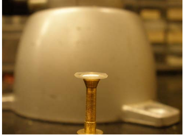
(b) A Lithium Niobate WGMR, 7mm in diameter ( Q \simeq 1.5 \times 10^8 )
