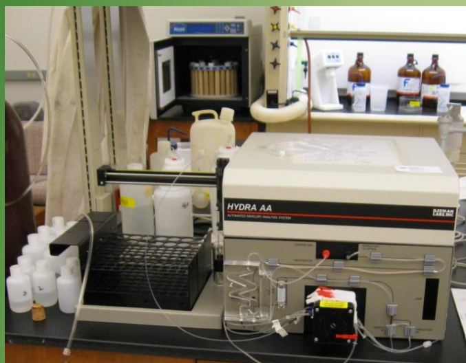
Automated mercury analyzer – based on atomic absorption from reduction of mercury via \text{SnCl}_2 (sub-ppb limits of detection)
